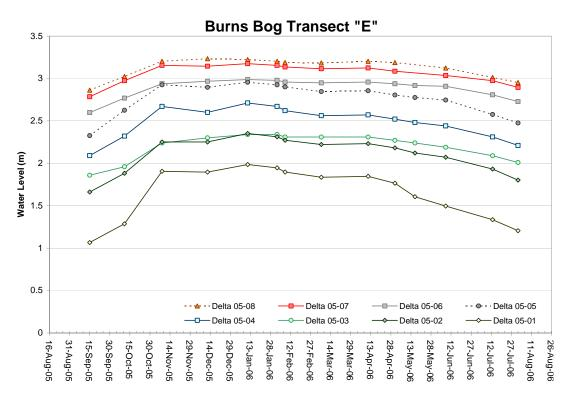
Figure 3 Seasonal and spatial variations in water levels along transect "E" of Burns Bog. The stations are ordered in relation to an axis along the radial flow pattern of the bog with Delta 05-08 being the innermost, and Delta 05-01 being near the bog margin within a few 10s of metres of a major peripheral drainage ditch system.
