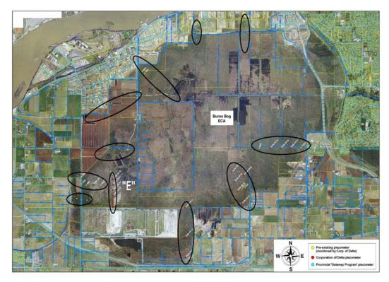
Figure 1. Burns Bog 2006. Blue lines and arrows indicate existing ditches and drainage directions. Red dots mark existing water level monitoring locations, and transects of sites are indicated by ovals. Note the transect labeled "E", considered in detail in the text.
