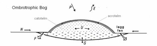
Figure 2. Morphology and hydrological relationships within an ombrotrophic bog. The thickness of the acrotelm is exaggerated in this view. Arrows indicate water fluxes: P, precipitation; N, surface water supply; U, lateral seepage in peat; E, evapotranspiration; F, surface water efflux; and G, exchange with deep groundwater (leakage) modified from Bragg (2002). The dashed area indicates the regional water table, and the dotted area the raised mound.
